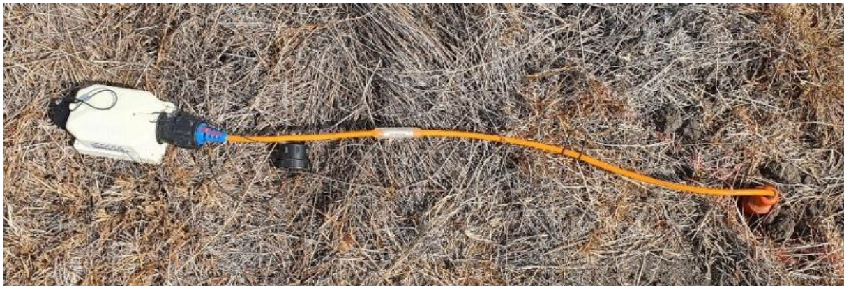
Figure 3-5: Wireless geophone ('node') with sensor installed in shallow hole
